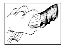
2. Begin by holding the firearm as shown. At the rearmost corner, cover the frame with the HANDALL. Make sure it is right side up. Look for the (up¹) inside the grip. Note: You may want to warm the HANDALL it the environment is cold for ease of installation. This can be done in hot or boiling water, or with a blow-dryer, etc. Warming the HANDALL will make it easier to stretch. On steel frame firearms, make sure the sleeve is completely dry so the firearm is protected against rust.
